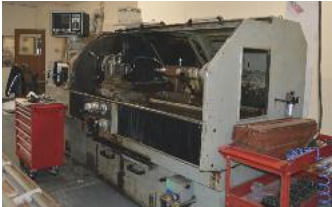
A lathe with a 'huge' 80 mm bore for producing 'Lazy S' clutch turns.
