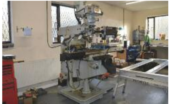
A CNC mill used to produce quality bespoke designs.
